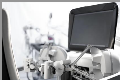
Surgeon console of the MiroSurge system with 3D display and input devices, capable of force/torque reflection
